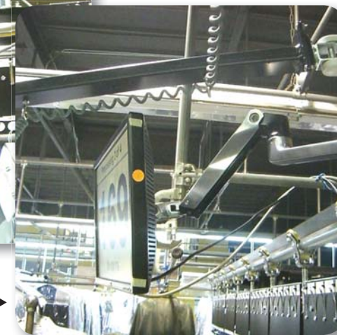
Shows a Scanner Kit includes overhead swivel arm, tool balancer, hand free scanner with 20' cable and necessary hardware.
